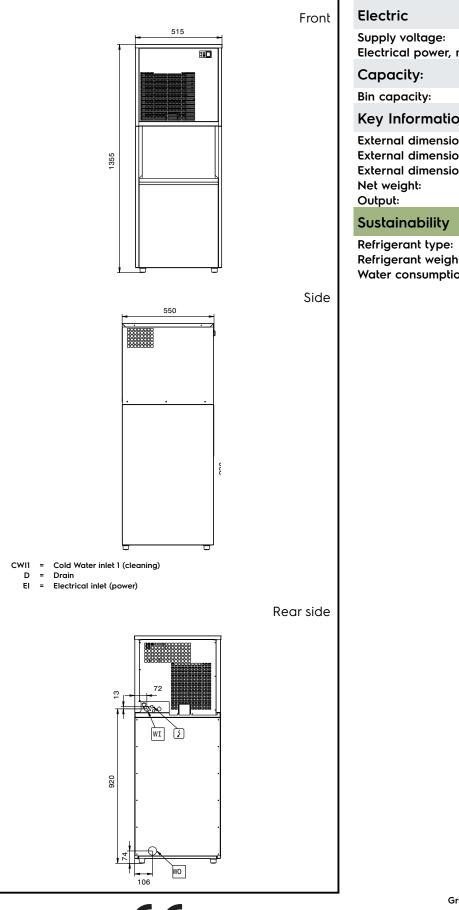
220-240 V/1N ph/50 Hz Electrical power, max: 0.65 kW 64 kg Key Information: External dimensions, Width: 515 mm External dimensions, Depth: 550 mm External dimensions, Height: 1460 mm 75 kg 178 kg/day R290 Refrigerant weight: 80 g Water consumption: 49.4 lt/hr
